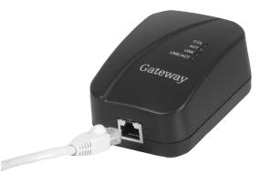
■ Plug the other end of the RJ-45 or USB cable into the computer
